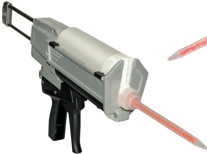
470 ml / 490 ml 10:1 Low-Resistance Manual Applicator Gun #11652 Use with Weld-On 11, 470 ml Cartridges Use Mixing Tip #13147
